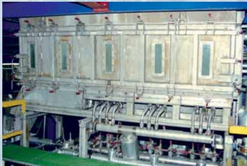
Granulator of pilot plant, capacity 150 mtpd
